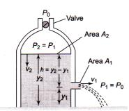
Fluid emerging from the hole is open to atmospheric pressure  $P_0$ , We take two points A and B at the top of the fluid and at the hole respectively. From Bernoulli's principle,
